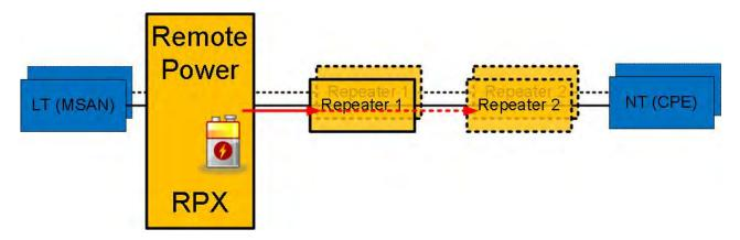
Feeding of up to 16 (32) repeaters with Remote Power Feeding Unit RPX16.
