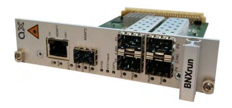
The BNXrun is a carrier-grade CPE device designed to match in a wide area of different applications. The BNXrun fits for the requirements of a Customer Premise Equipment (CPE) in a FTTH-scenario as well as a Network Interface Device (NID) for other FTTx-scenarios. The BNXrun is designed to enable Layer2 and Layer3 business services, including an outstanding support for clock distribution and time synchronisation to the provider's edge.
