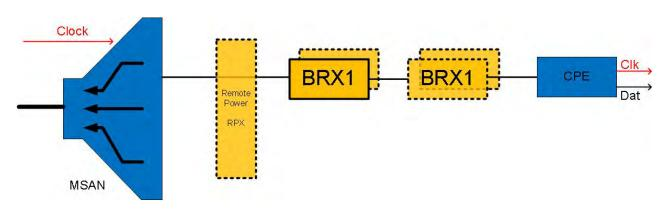
BRX1 used as line extension from MSAN to EFM CPE. Remote power of BRX, line bundling and doubled extension with two regenerators is possible.
