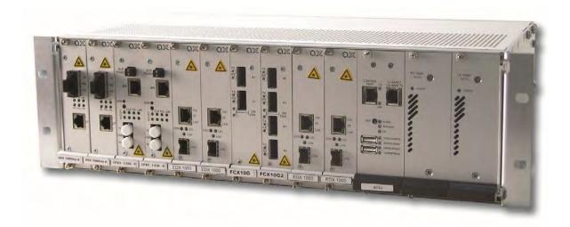
The SHX-Family offer a simple and flexible solutions to build a standalone unit using one of arcutronix 3RU rack mount cards. An integrated wide-range power supply gives the opportunity to feed the SHX either with 110/230VAC mains or 48VDC input.
